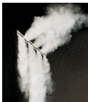
Air jet pattern of WSD above: horizontal air jet left: one jet inclined upwards and one jet downwards
