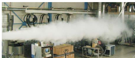
Air jet pattern of DW-V2
