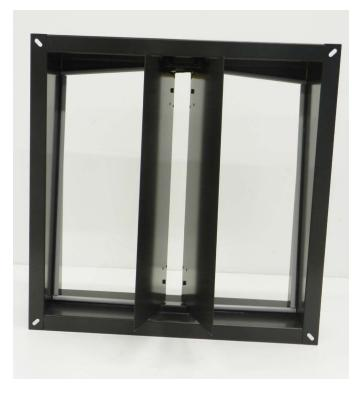
Due to space constraint, backdraft dampers are frequently installed closed to fan discharge in ventilation system causing rattling noise and damage to the blade, blade linkage and its bearings. Our engineer at OLS have produced a completely new version of the backdraft damper that is fail-proof from air turbulence and does not cause rattling noise under turbulence flow.
