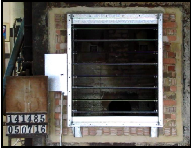
View of the unexposed side of wall mounted damper before testing.
